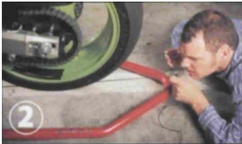
Now, pull the string to, and alongside, the forward sidewalls of the rear tire until it is just touching. Sight along the string and make sure that the gaps at the very rear of the front wheel are equal. Check the gaps
